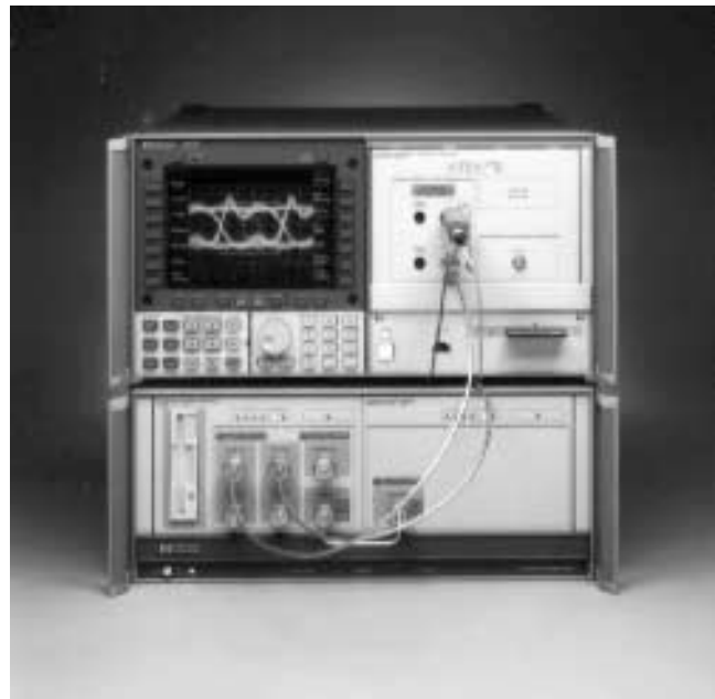
Fig. 4. Photograph of the HP 71501A eye diagram analyzer with an HP 71603B pattern generator system.
